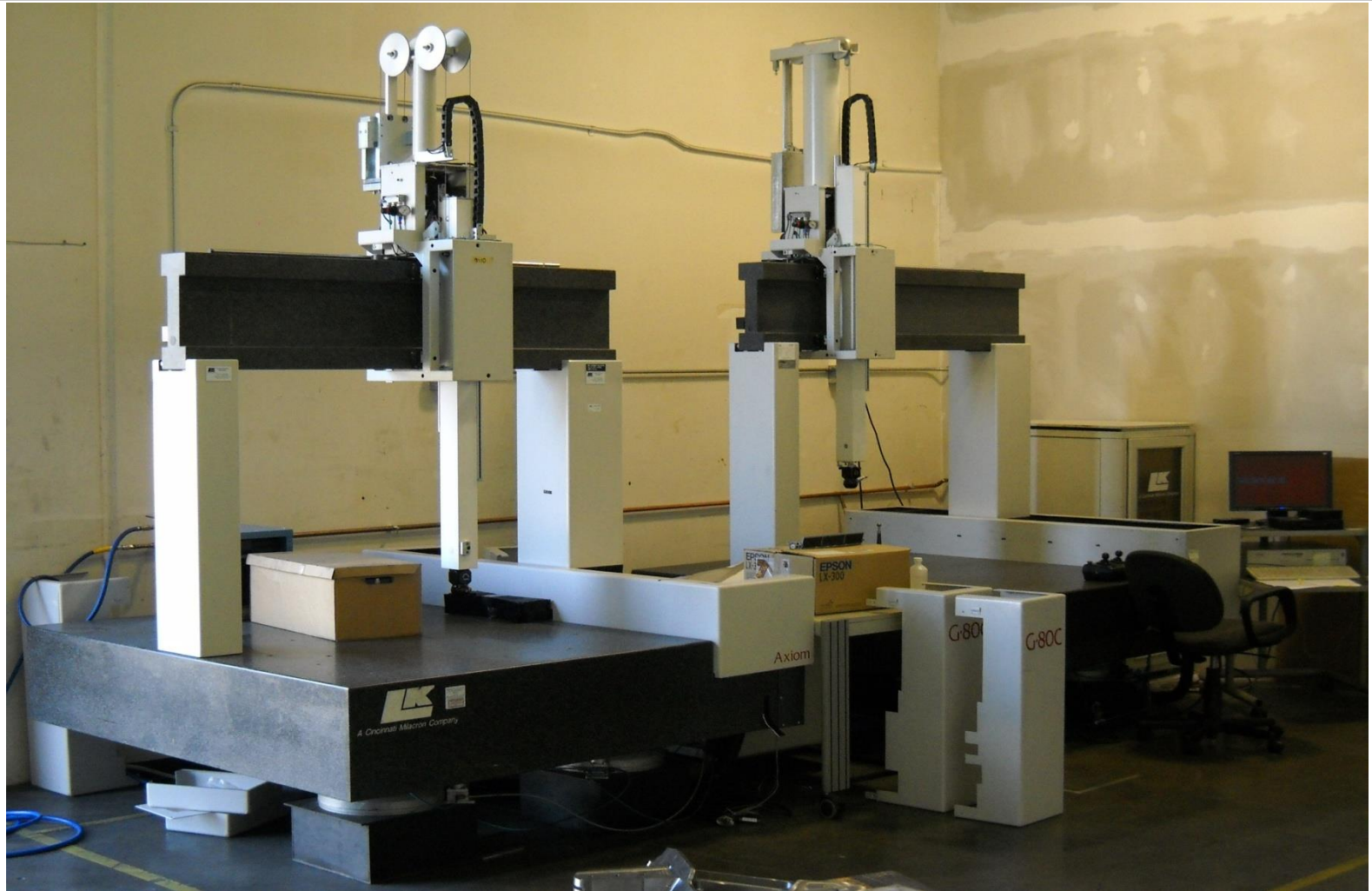
Dual LK G-80C CMM's 40" x 38" x 29" w/ Renishaw PH9A motorized heads
